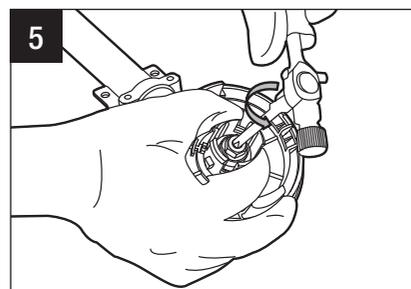
4. Hold the spool base and pull it straight out from the motor shaft (Fig. 6).
